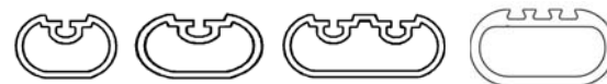
Polished and Bright Dipped Oval Tubes with slots left to right: 25-BD-250, 25-BD-255, 25-BD-212, 25-BD-206
